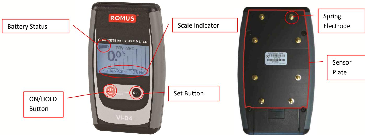
Picture below illustrates meter's front and back panel with most important elements marked:
